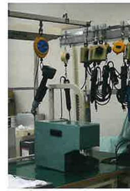
Tool Hanger The tool can be hung on the balancer.
